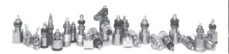
P6 series switches are sealed against immersion and corrosive atmospheres. These switches are designed for rugged duty both mechanically and electrically. A one-piece stainless steel or nickel plated brass housing, sealed at the plunger with an O-ring seal and at the base with a glass-to-metal header option provides true environment-free sealing to comply with MIL-PRF-8805/39, MIL-PRF-8805/40, MIL-PRF-8805/43, MIL-PRF-8805/100 and MIL-PRF-8805/104. Most case parts are grounded for EMI reduction.
